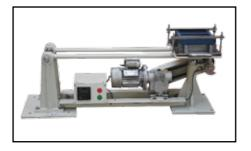
This machine consists of a mould table which is seated on a rotating cam driven at 60 rpm and features push button start/stop control, and automatic stop control at the end of test.
