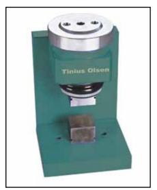
This attachment is designed for testing the compressive strength of mortar cubes, or the block resulting from a flex test specimen. This attachment must be used with the appropriate compression platens.
