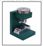
This attachment is designed for the flexural testing of 40 x 40 x 160 mm mortar cubes.
